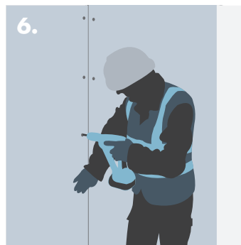
6. Fixing Knauf Soundshield Plus to the frame.
