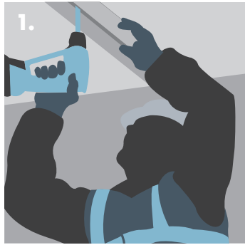
1. After fixing the head track, the floor track should be positioned by using a vertical stud and a laser/spirit level.
