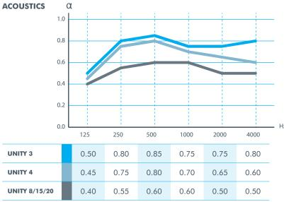
CONSTRUCTION 200 mm suspension, no mineral wool
