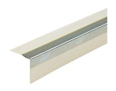
Knauf Las Vegas B2 Internal Bead is a paper faced internal bead to create 90° outside corners on any thickness of Knauf plasterboard. For indoor use only.
